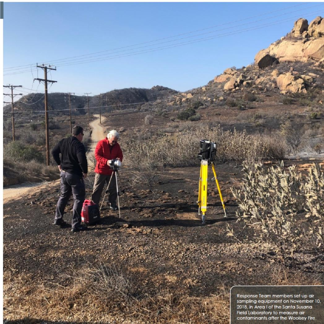
Response Team members set up air sampling equipment on November 10, 2018, in Area I of the Santa Susana Field Laboratory to measure air contaminants after the Woolsey Fire.
